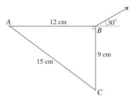
A uniform right-angled triangular lamina ABC with sides AB = 12 cm, BC = 9 cm and AC = 15 cm is freely suspended from a hinge at its vertex A. The lamina has mass 2 kg and is held in equilibrium with AB horizontal by means of a string attached to B. The string is at an angle of  $30^{\circ}$  to the horizontal (see diagram). Calculate the tension in the string.
